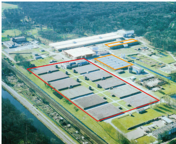
Figure 33 - Difference in surface area between rapid filtration (orange) and slow sand filtration (red)
