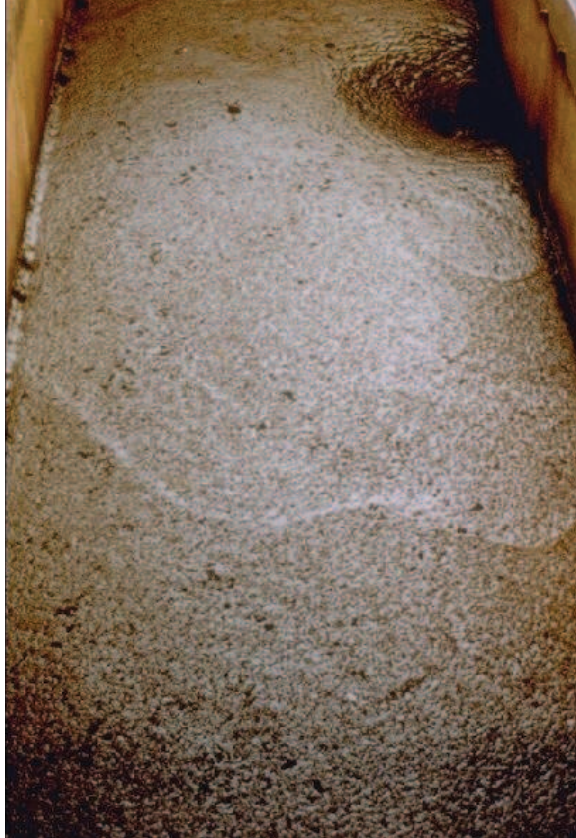
Figure 20 - Result of a poorly designed filter bottom
